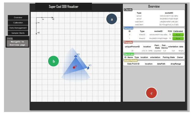
Figure 3. The visualization and prototyping tool for the *SoD-Toolkit*. (a) The tracked environment, (b) Entities tracked in the environment, (c) List of available entities and their current state, as well as clients currently connected in the environment.
