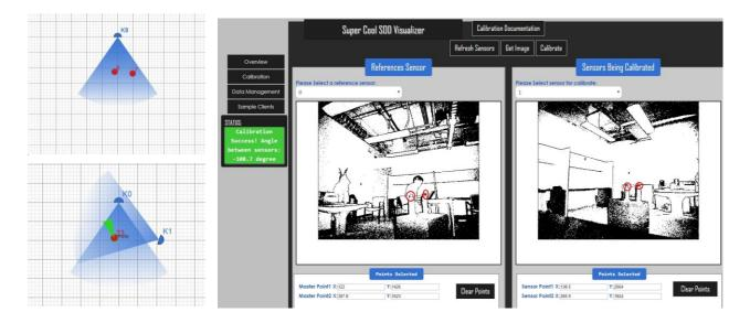
Figure 4. Sensor Fusion using multiple Kinect sensors. (a) 2 uncalibrated Kinect sensors (overlapping) showing skeletons tracked in the environment. (b) Interface for calibration. (c) Properly calibrated environment with overlapping Kinect areas.
