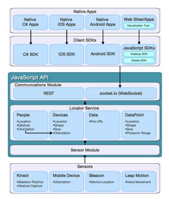
Figure 2. An overview of the architecture of the SoD-Toolkit
